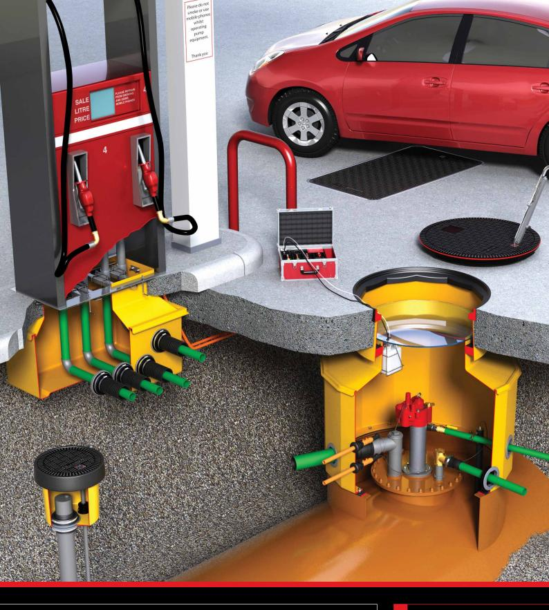
GRP Composite Manhole Covers & Underground Containment Systems
