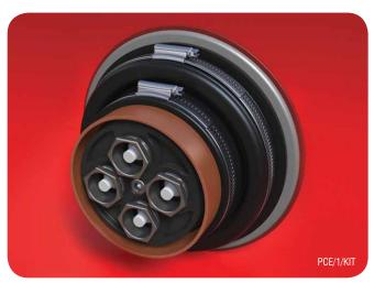
Fibrelite's range of pipe and cable entry kits offer a unique design allowing a single hole installation. No additional screw holes need to be drilled. This provides the installer with a quick and easy installation and minimises potential leak paths through the sump wall. The pipe sleeves are made from a fuel resistant nitrile grade or viton rubber and the bellowed design facilitates movement with changing ground conditions.
